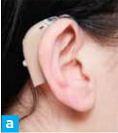
Behind-the-ear (BTE) hearing aids usually have an earmould which sits inside your ear. The hearing aid rests behind your ear and a plastic tube connects it to the earmould.
